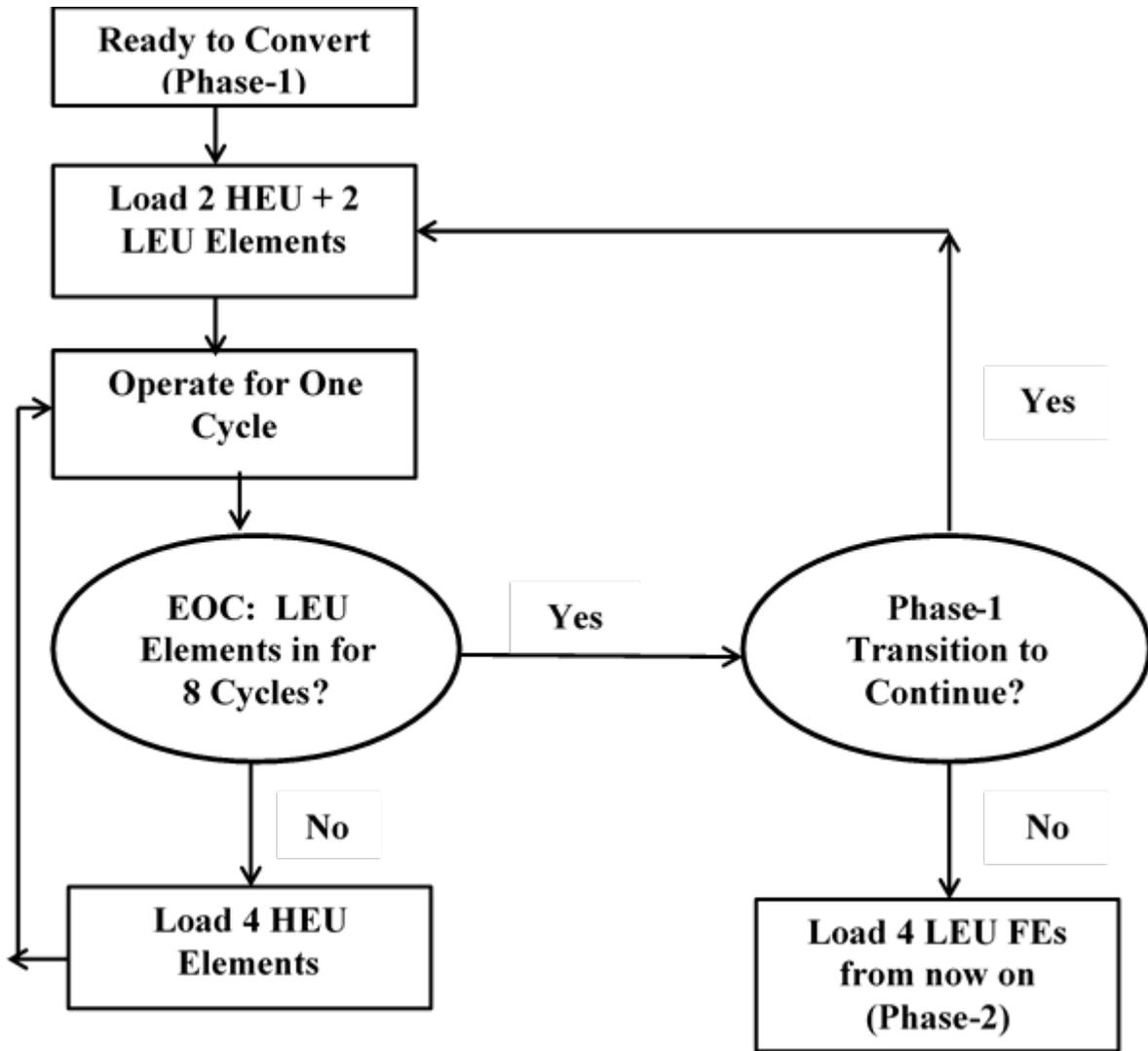
**Figure 2. Flow Diagram for Transition from HEU to LEU Fuel**
