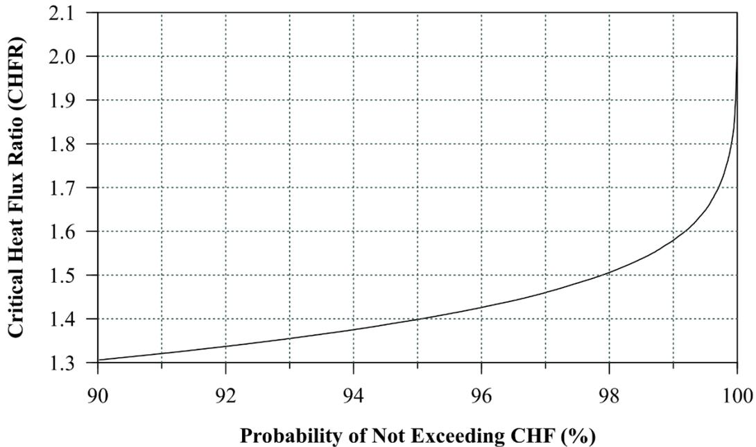
**Figure 3. Cumulative Distribution Function for Critical Heat Flux Ratio**
